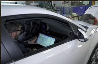
Chassis dyno testing for vehicle emissions and fuel efficiency
